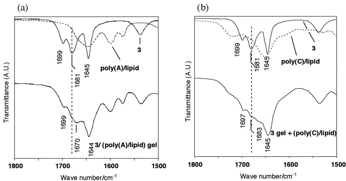
**Fig. 7** (a) ATR-FTIR spectra of xerogel obtained from **3** gel (solid line), poly(A)-lipid (dotted line) and **3**-(poly(A)-lipid) gel (lower part). (b) ATR-FTIR spectra of xerogel obtained from **3** gel (solid line), poly(C)-lipid (dotted line) and **3** gel + (poly(C)-lipid) (lower part).
