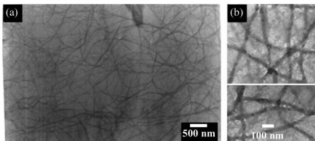
**Fig. 4** (a) TEM image obtained from **1**–poly(A) gel (5.0% (w/v), [adenine base] : [**1**] = 0.7) gel and (b) its magnified image.
