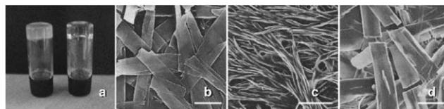
**Fig. 8** (a) Photo image of gel sample created by **2** gel (left) and **2**-(poly(A)-lipid) gel (right). SEM images of (b) **2** gel, (c) **2**-(poly(A)-lipid) gel and (d) **2** gel + (poly(C)-lipid); [adenine base or cytosine base] : [thymidine] = 1.0. All scale bars indicate  $5\text{ }\mu\text{m}$ .
