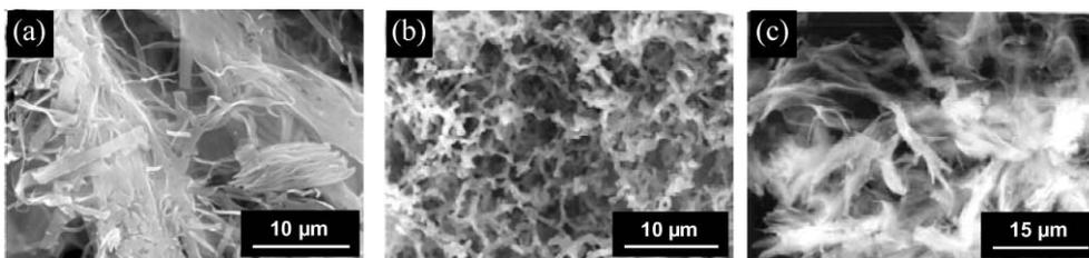
**Fig. 10** SEM images of xerogel obtained from (a) only **3**, (b) **3**–(poly(A)–lipid) ([adenine base] : [**3**] = 1.0) and (c) **3** gel + (poly(C)–lipid) ([cytosine base] : [**3**] = 1.0).
